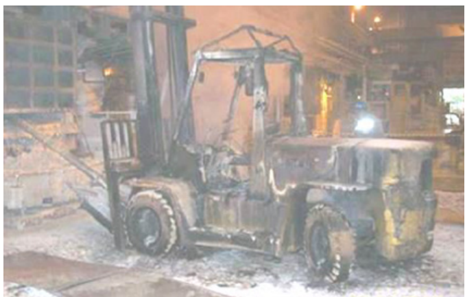
31.1 Figure 2 – Fork Truck Following a Furnace Explosion
