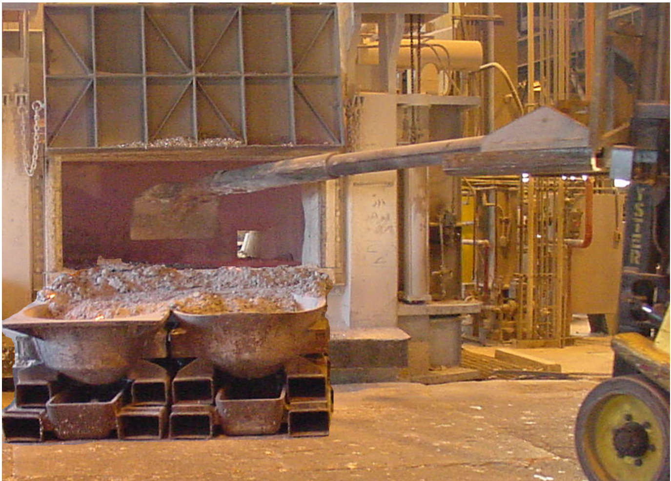
16.4 Figure 1 – Skimming Dross from a Furnace by Mechanical Skimmer
