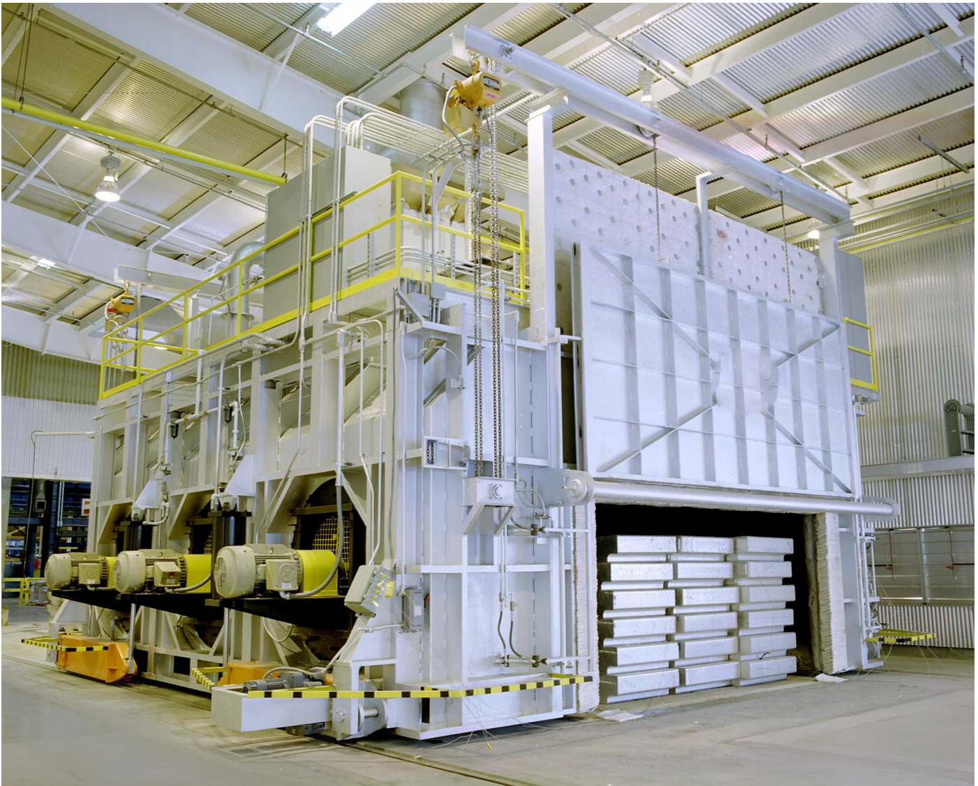
14.1 Figure 1 - Example of a commercially available sow drying system. The system shown is a natural gas fired dryer with positive pressure and recirculation fans.
