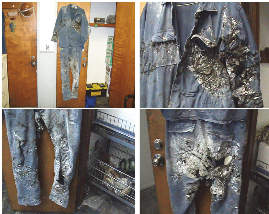
11.3 Figure 1 - FR garments worn by employee exposed to molten metal from a drain pan explosion. Use of FR garments minimized the extent of burn injuries.
