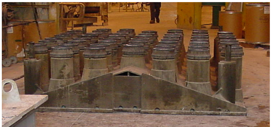
9.3.4 Figure 1 – Billet Base Plate with Starting Blocks
