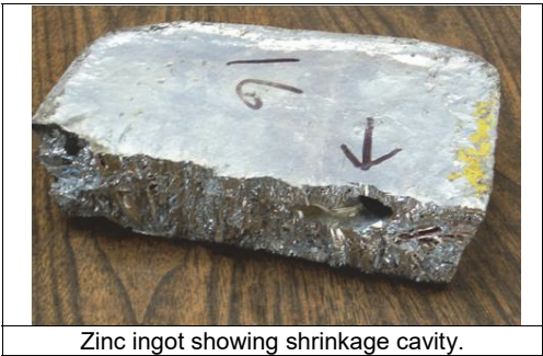
13.1.3 – Figure 2 Example of a zinc ingot with a shrinkage cavity
