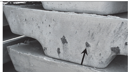
Flux salts imbedded in the end surface of RSI
