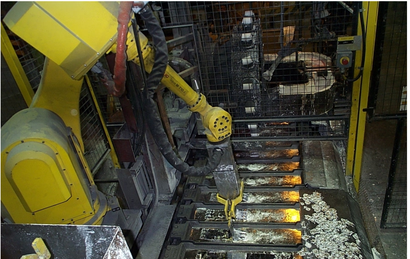
8.3.6 Figure 1 – A Robotic Pig Ingot Casting Machine with Skimming and Metal Filling Control
