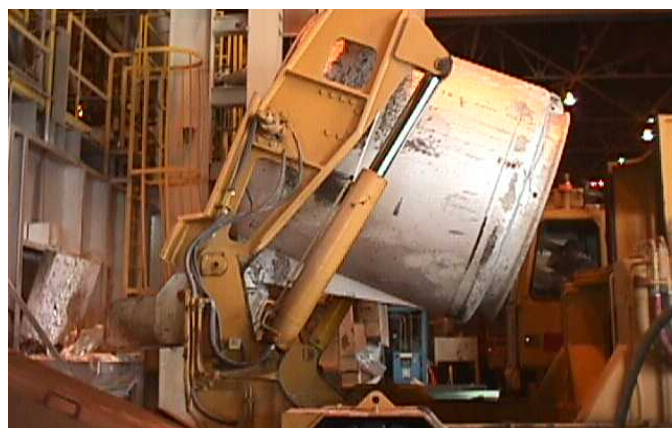
8.1 Figure 1 - Charging a Furnace from a Transfer Crucible
