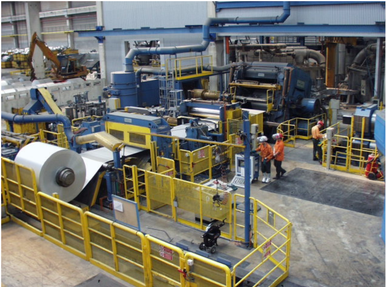
8.3.5 Figure 1 – One Type of Continuous Strip Casting Machine
