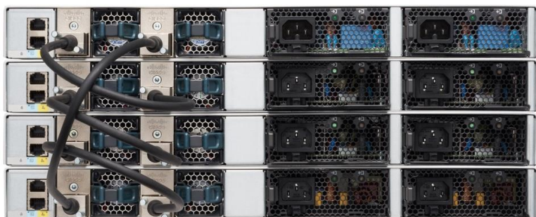
Figure 4. Cisco Catalyst 9200 Series Switch stacked units
