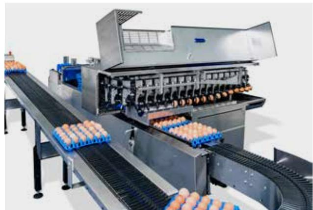
After the arrival of the 6th egg in the dropset, the Farmpacker places all the eggs into a tray in one cycle. The result of the concept of individual egg handling is:
