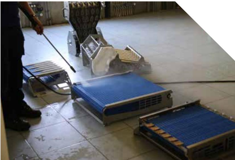
All the egg-touching parts of the Mopack150 can be removed from the machine for cleaning outside egg packing room. The main advantage of this construction method is that this allows for a hygienic and clean packing process. This will ultimately result in more grade-A eggs being supplied to your egg retailer.
