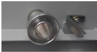
Lock installed in internal part of door
